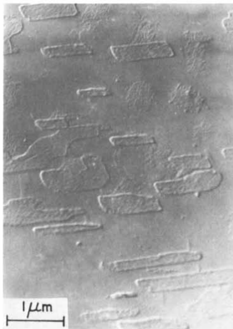
Figure 2. DMDA polymerized on KBr and deposited from a wt% toluene solution at 78 °C.
